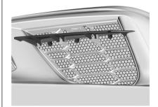
For vehicles with the optional Grille Screen Guards (VWE), remove them for track events when the ambient temperature reaches 32° C (90° F) or higher. See your dealer for complete procedure.
