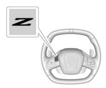
To activate Z Mode, press the Z Mode button on the steering wheel. To deactivate, select a different mode through the DMC knob, or press the Z Mode button on the steering wheel.
