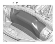
5. Remove the rear compartment access panel screws (2) and panel (1).
