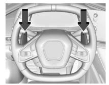
With the transmission in D (Drive), press the M (Manual Mode) switch on the center console to enter Manual Mode. Use the paddles on the steering wheel to manually upshift or downshift the transmission. The right + (plus) paddle upshifts, and the left – (minus) paddle downshifts.
