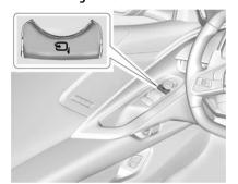
If equipped, press □₄ to power fold the mirrors. Press □₄ again to unfold.
