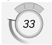
The electric power indicator gauge is in the middle of the display to the left of the speedometer, and is shown in the Stealth mode.
