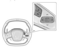
Press < or > to access the cluster applications. Use the thumbwheel to scroll \( \script{\script{or V}}\) through the list of available features. Press the thumbwheel to select. Not all applications will be available on all vehicles.
