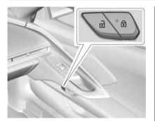
The passenger power door lock switch can also be used to lock or unlock the doors.
