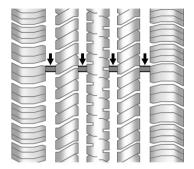
Treadwear indicators are one way to tell when it is time for new tires. Treadwear indicators appear when the tires have only 1.6 mm (1/16 in) or less of tread remaining. See *Tire Inspection* ♀ 305 and *Tire Rotation* ♀ 305.
