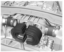
8. Remove the air cleaner filter(s) (top image LT2 engine) (bottom image LT6 engine).
