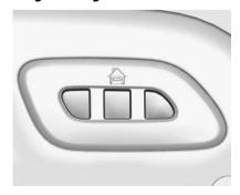
If equipped, these buttons are in the sunshade. This system can replace up to three remote control transmitters used to activate devices such as garage door openers, security systems, and home automation devices. These instructions refer to a garage door opener, but can be used for other devices.
