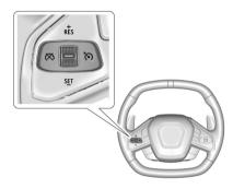
্ধৈ: Press to turn cruise control on or off. A white cruise control indicator light comes on in the instrument cluster when cruise is turned on.
