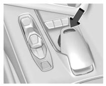
To activate My Mode, Weather, Tour, Sport and Track mode, turn the DMC knob on the center consoleto make a mode selection. When a mode is selected, an indicator will come on in the instrument cluster and stay on. See "E-Ray – EV Drive Mode Activation" later on in this section for details on activating EV drive modes.
