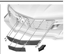
If equipped, remove the front license plate and bracket (if installed) and remove the front aero covers before track use. See your dealer for complete procedure.
