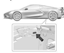
Use only a service jack with a lifting pad diameter of 64 mm (2.5 in) or smaller, and thick enough to make sure the jack does not contact the vehicle body.
