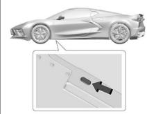
Use only a service jack with a lifting pad diameter of 64 mm (2.5 in) or smaller, and thick enough to make sure the jack does not contact the vehicle body.
