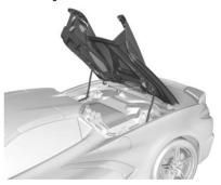
5. Hold ڪے until the tonneau cover is completely opened. The turn signals will flash once
