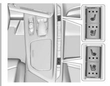
If equipped, the buttons are near the climate controls on the console. To operate, the engine must be running.
