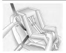
7. To tighten the belt, push down on the child restraint, pull the shoulder portion of the belt to tighten the lap portion of the belt, and feed the shoulder belt back into the retractor. When installing a forward-facing child restraint, it may be helpful to use your knee to push down on the child restraint as you tighten the belt.
