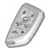
Press to lock both doors and the fuel door. The turn signal indicators may flash and/or the horn may sound on the second press to indicate locking. See "Remote Lock, Unlock, Start" under Vehicle Personalization ⇔ 116.
