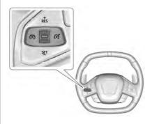
$\infty$ : Press to turn cruise control on or off. A white indicator comes on in the instrument cluster when cruise is turned on. **+RES** : If there is a set speed in memory, press briefly to resume to that speed or press and hold to accelerate. If cruise control is already engaged, use to increase vehicle speed.
