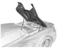
Hold the tonneau cover is completely opened. The turn signals will flash once.
