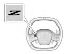
To activate Z-Mode, press the Z-Mode button on the steering wheel. To deactivate, the driver can either select a different mode through the DMC knob or press the Z-Mode button on the steering wheel. When Z-Mode is deactivated through the Z-Mode button, DMC is always set back to Tour Mode.
