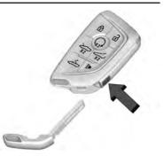
1. Press the button on the side of the remote key and pull the mechanical key out. Never pull the mechanical key out without pressing the button.
