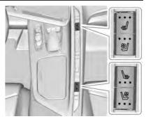
If equipped, the buttons are near the climate controls on the console. To operate, the engine must be running.
