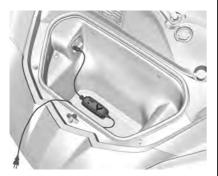
Some vehicles have a battery maintainer package. Follow the instructions provided with the battery maintainer package to keep
