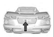
Use the mechanical key in the backup key cylinder behind the license plate to manually open the hatch/trunk. The license plate must be removed.
