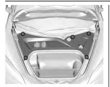
2. Release the five clips and remove the outer cover.
