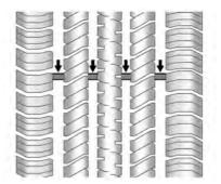
Treadwear indicators are one way to tell when it is time for new tires. Treadwear indicators appear when the tires have only 1.6 mm (1/16 in)
