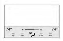
The climate control status display appears briefly when the center stack climate controls are adjusted.
