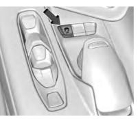
The TCS/StabiliTrak/ESC button is on the center console.
