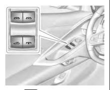
Press **F** to lower the midglass. To provide wind block, the midglass will not lower completely. The midglass will also lower automatically when lowering the convertible top.
