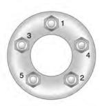
Tighten the wheel lug nuts firmly in a crisscross sequence. See *Capacities and Specifications* ⇔ 300.
