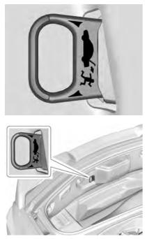
There is a glow-in-the-dark emergency hatch/trunk release handle on the inside back wall of the storage compartment. This handle will glow following exposure to light. Pull the release handle to open the hatch/trunk from the inside.
