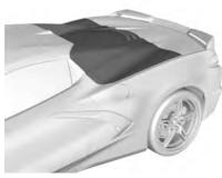
Hold the tonneau cover is completely closed. A chime will sound, a DIC message will display, and the turn signals will flash once.
