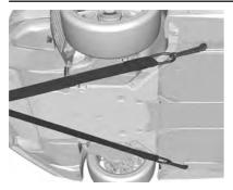
The vehicle is equipped with slots that are located underneath the vehicle rearward of the front tires. These can be used to pull the vehicle onto a flatbed car carrier from a flat road surface. Do not use the tow eye to pull the vehicle from snow, mud, or sand.
