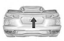
Press the hatch/trunk release touchpad to open the trunk if the remote key is within 1 m (3 ft).
