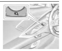
If equipped, press ⊡₁ to power fold the mirrors. Press ⊡₁ again to unfold.
