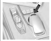
To activate My Mode, Weather, Tour, Sport and Track Mode, turn the Driver Mode Control (DMC) knob on the center console to make a mode selection. When a mode is selected, a unique and persistent indicator will be display in the driver information center (DIC).
