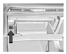
The PDR records video, audio, and vehicle data. This data is stored on a removable SD card in the glove box.
